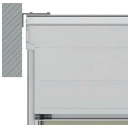
Installation laterally on a wall or in a niche using the 200 x 100 x 10 x 140 mm angle bracket
