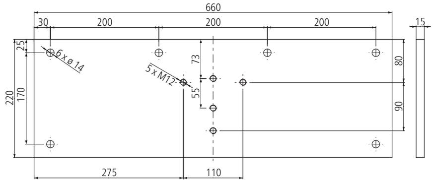
Position of the mounting plates using the Opal Design II 500 x 300 cm\* as an example.
