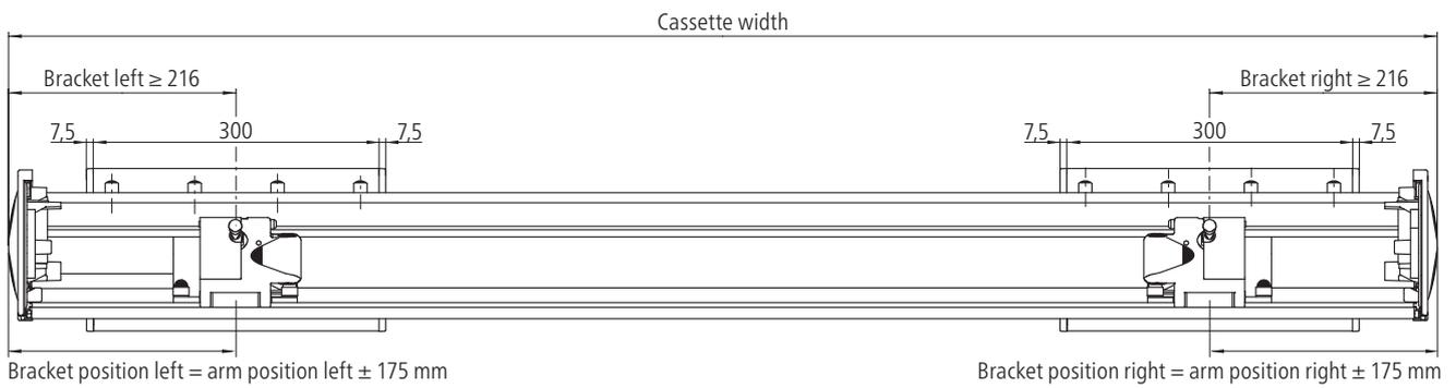
**Wall bracket 300 mm (left and right) with wall bracket 150 mm (centre)**
