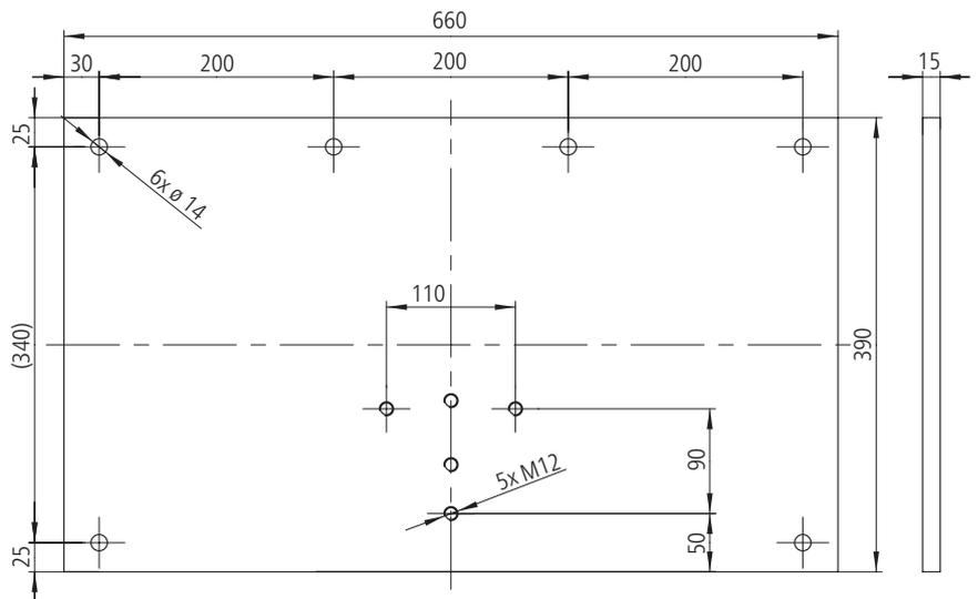
Position of the mounting plates using the Opal Design II 500 x 300 cm\* as an example.
